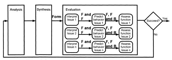
Figure 1, Model of design evaluation process. The synthesis step produces a description of form. During evaluation, the form must be interpreted to associate function with the form for each issue. For each function, behaviors must be predicted using the form. Finally, the functions are assessed by examining the behaviors. The result is a determination of whether the potential solution is successful.
