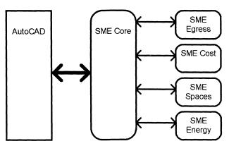
Figure 2, Semantic Modeling Extension system architecture. The components shown with rounded rectangles were programmed with Kappa. The large arrow symbolizes that the link between these components is instituted permanently for a session with SME. The small arrows indicate links that may dynamically be created or severed during a session to accommodate changing needs for evaluations.
